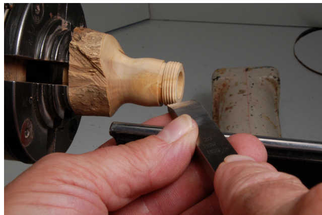
Begin chasing the external threads with the tool starting at a 45 degree angle
