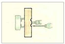
You can cut a recess on the lathe with a parting tool while holding the blank securely with the tailstock. Jamming the blank against the open jaws of a chuck works very well. Be sure to center the blank first.
