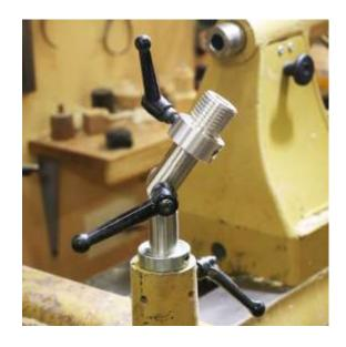
Loosening the upper lever allows rotating the piece to work on different corners and edges without having to juggle the piece with two hands.
