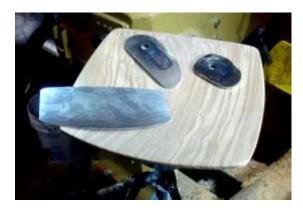
A larger curved scraper will quickly smooth away ripples in the dish and leave the surface very smooth. Always scrape downhill!
