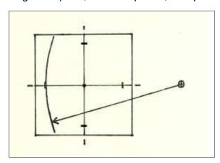
Anchor the center of the square to a work surface with a pushpin through the center.
