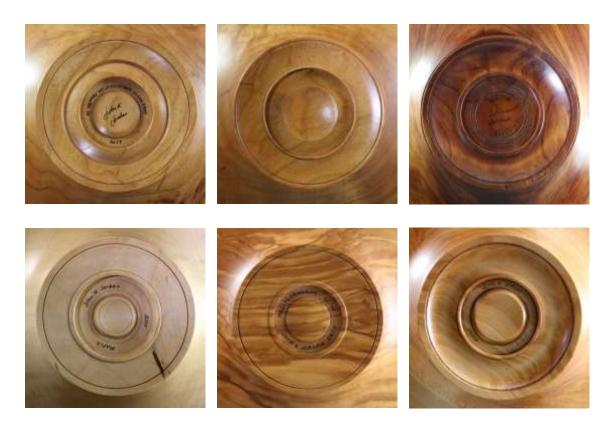
Now shape the bottom outside the base ring to create a continuous smooth curve from the base to the corners of the rim. A small bowl gouge is excellent but the small Hunter Hercules tool is my favorite. Tools must be SHARP when turning air.
