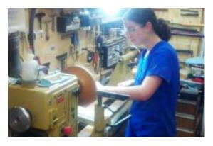
Dish the top, being aware of the recess in the bottom. I like a smooth curve, turning the wings and outer areas parallel to the curve of the bottom. This will make the rim the same thickness all the way across each side. If the dish is too shallow the rim will be thicker in the center.
