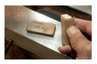
Two things help reveal surface defects such as tool marks and sanding scratches. First, use a bright light at a glancing angle. Second, wipe naptha on the surface with a paper towel and examine the surface at different angles.
