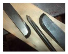
The curve lets only a small part of the edge touch the wood and the flat I grind at the end is important. Grind the bottom bevel last.
