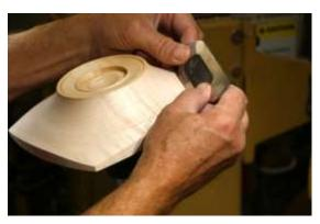
The smaller scrapers are excellent for the bottoms of these little platters. A flat or gently curved edge can be used on the curves of the bottom and to remove all tool marks from the wings.
