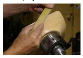
Shape by hand with files, sand paper, or my favorite, sanding sticks. Minor chips on the edges can be removed. The rim might be rounded, angled, or thinned. This is also the best time to round the corners slightly if desired.
