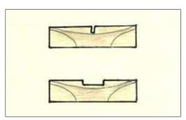
To hold the blank by the top I usually use a screw chuck since it involves simply drilling a hole. I use the Glaser screw chuck.
