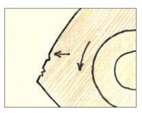
At the very edge the gouge is pushing unsupported fibers into the air and can throw chips off the edge of the rim.
