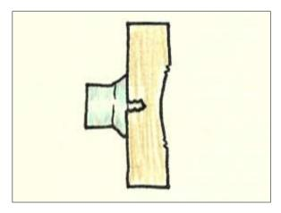
I like to create a narrow ring just inside the base diameter because I like the way it looks. I use a parting tool to cut a second angled groove to define the inside of the ring.
