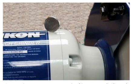
To the left is an example of an inexpensive grinder with stock wheels after balancing. That nickel has been sitting on the running bench grinder for over 10 minutes! It took only 30 minutes to true the wheels using the Don Geiger method.
