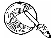
Top or blade nose touches bottom or side of kerf during reinsertion
