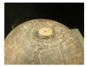
25. With a scrap mounted in the chuck, cut a taper that will fit into the neck of the vessel. Now the vessel can be remounted using the center marked on the piece attached to the plug to align the live center. Now cut a second grove beside the glue line and work both until they match. Remove the vessel, sand the bottom, sign and apply your favorite finish.
