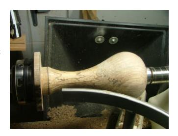
**17.** Slide the tailstock back and use a small gouge to slightly taper (about 5°) the 1 ½" entry hole to accept the plug. The 1/8" left on the base when parted should be left at this point.
