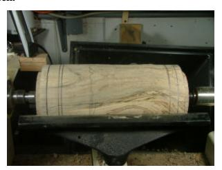
**3.** Mount spur end (vessel base) in chuck. Bring up tailstock to maintain center and apply pressure when tightening chuck. At chuck end mark the tenon between #1 & #4 jaw. Align this mark with the toolrest and transfer a mark to the tenon on tailstock end. (This becomes important in matching grain in bottom plug.)
