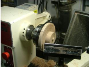
19. Once the fit is good, we are ready to glue it in. Now is where those marks we made on the two tenons help us to line up the grain in the plug with the vessel Apply glue (white glue not CA) to tenon and base and bring up the tailstock with a cone center in the ½" hole to achieve proper alignment and hold the piece until the glue sets (preferably overnight).
