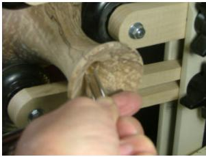
**22.** The last step is to remove the plastic wrap and the three strips and part off the vessel. Leave about 1/8" of the base plug to be taken off with a sanding disk.
