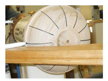
11. Use a piece of ½" tape (or regular masking tape) to sketch the spiral to be carved. I prefer to use tape, as I can adjust it and not have to erase lines when I change the shape of the spiral. Tape one or more spirals until you get one that you like. Then remove the tapes spirals that you didn't like and keep the remaining one that you did like. Once you have the one that you like, mount the bowl back on the lathe.
