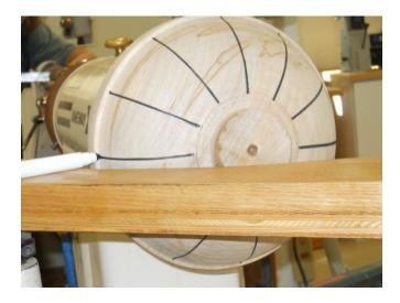
10. Now we will start to draw out the curve for our spirals. Take the bowl off of the lathe, but don't take it out of the chuck. If you leave the bowl in the chuck it will remain centered when you put it back on the lathe. Place the bowl in the chuck upside down so it is resting on a solid, stable work surface. When you are working on the bowl, you will see the bottom of the bowl. See picture below.
