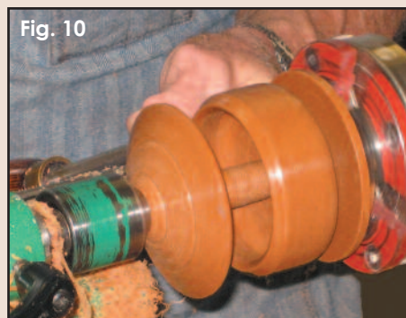
Fig. 10 Form the bottom with the 3/8" gouge.
