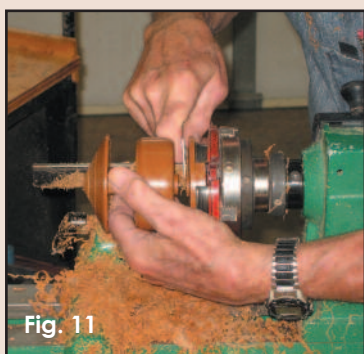
Fig. 11 Part the blank off the lathe.
