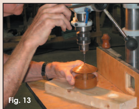
Drill a hole for the screw eye on the drill press.
