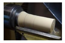
I use my parting tool to cut a line at  $2\frac{1}{2}$ " down to 1". Then I move up to  $3\frac{1}{2}$ " and cut another groove down to 1". Then clean up in between these 2. This will be the head. Now turn the skirt all except for the very top.
