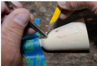
The thickness of the pencil line makes it really close to ¼". I cut the hole with my Dremel.
