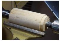
Mount this in the chuck and then turn it down to  $2\frac{1}{2}$ " in diameter. Then mark a line  $2\frac{1}{2}$ " from the end and another one  $3\frac{1}{2}$ ". This is for the head.
