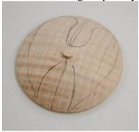
To shape the wing I use a flat board with a V notch clamped to the work bench. I use either a coping saw with a fine tooth blade or a jewelers saw with a blade that is appropriate.
