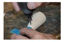
I test fit and cut more until the tenon fits. Then I simply glue it in with medium CA or fast set epoxy.
