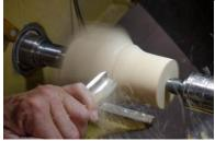
I mount it between centers and round it off and then turn a small tenon for my chuck on one end.
