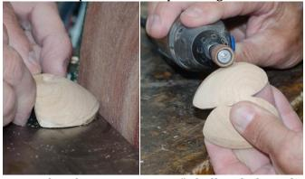
To glue the wing I cut a  $\frac{1}{4}$ " shallow hole in the Angel using my Dremel. I use a  $\frac{13}{16}$ " drill bit and set the shank exactly where I want the hole. Then I simply draw around this.
