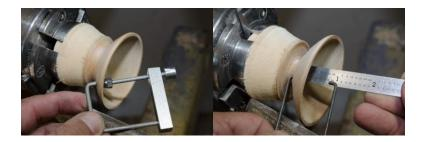
I use a parting tool to cut down to about ½" and then cut stair steps so I very roughly shape the outside of the bowl. Then use the Hunter tool cutting from tenon
