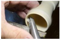
I can usually get the inside clean enough to sand with 220 grit or finer depending on the wood. Since I sign the inside with a permanent marker I like this to be sanded to at least 600 grit.
