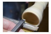
You could probably leave it like that or start your sanding there but I like to use a Hunter straight ornament hollowing tool to clean up the inside. I cut from the center out in a bevel rubbing cut and then use the tool with the cutter facing the wall and do a shear cut out to the bottom.
