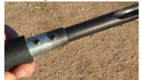
The 5/8" bowl gouge in the pipe handle using set screws to hold it in.
