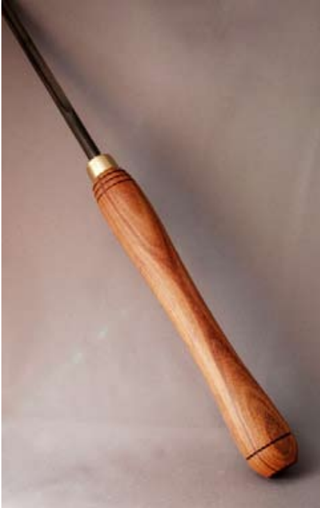
3/8" detail gouge mounted in handle using a 1/2" brass coupling nut for the ferrule.
