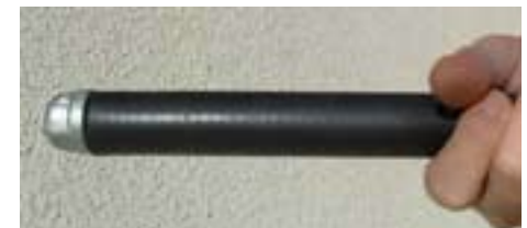
The metal handle with the end cap and covered with dishwasher hose. If the handle isn't heavy enough for you just add some lead shot or BBs.
