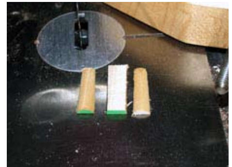
Results of the ripping cuts in the dowel. Discard the center piece and use the two half-round shims to give a good fit in the handle.
