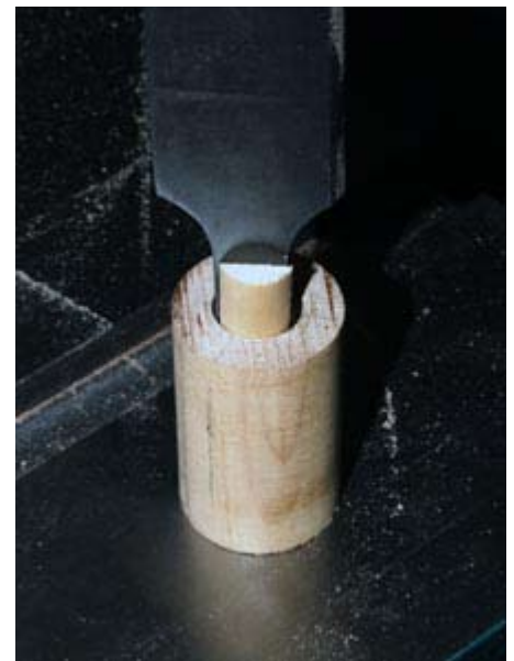
This is a mock-up I use to test the size of the shims I cut on the bandsaw. You may have to make several cuts to get them just right. The stock is a small piece of 1 1/4" maple dowel with a 5/8" hole drilled to a depth of 1 1/2".
