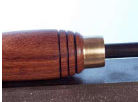
This is a close-up view of the spindle detail gouge with a 3/8" shaft mounted to the handle with a 1/2" brass coupling nut.
