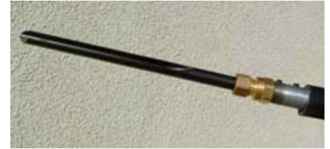
The 1/2" bowl gouge in the pipe handle using the 3/4" compression fitting.
