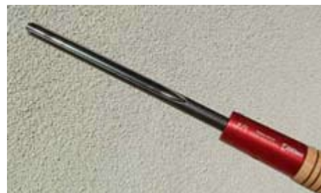
The 1/2" bowl gouge in the Thread-Lok Ferrule.
