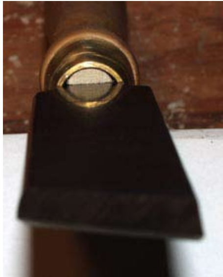
View of the finished handle for the skew showing the half-round shims used to strengthen the handle at the ferrule. The epoxy hasn't been added so as not to obscure the view of the shims.
