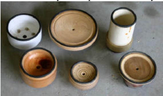
These are all homemade chucks. They have a rubber seal on the lip of the chuck to seal the vacuum from leaking.
