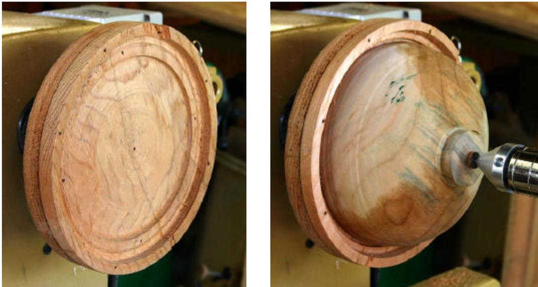
You can often use this disc of wood several times by turning different size grooves for the bowls. When you cut it down to the point that the screws from the faceplate are close simply true up the surface and glue another scrap of wood on top.
