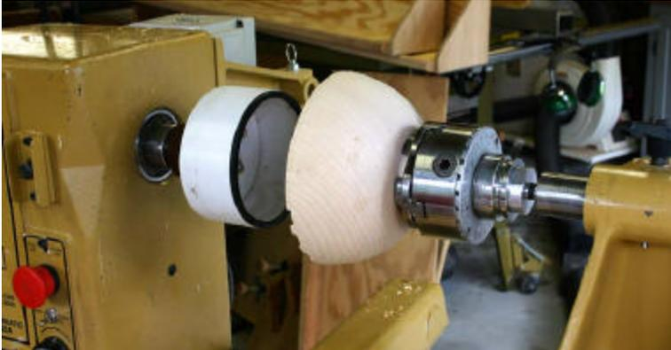
You simply mount the bowl and chuck on the tailstock adaptor and then slide the bowl up to the vacuum chuck. Then you turn on the vacuum pump and then remove the chuck from the bottom of the bowl.
