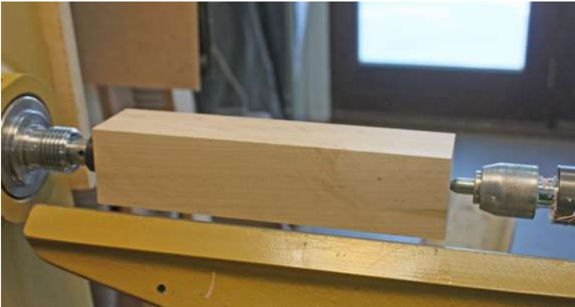
1. Blank mounted between centers
