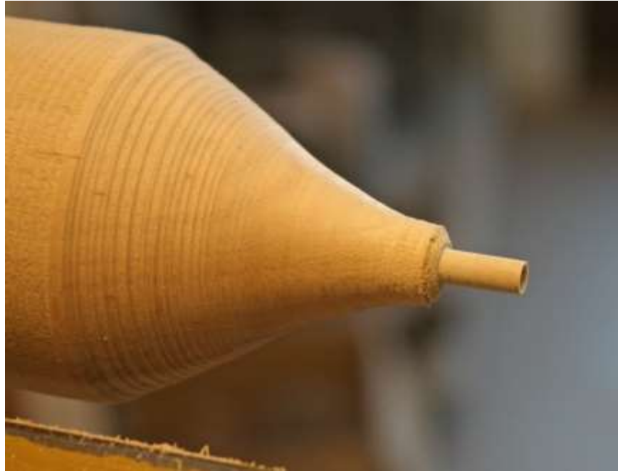
6. end of blank turned to diameter of small supporting cup
