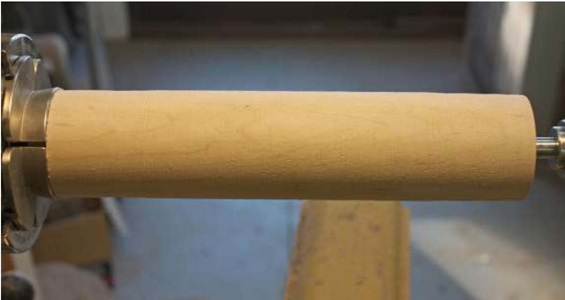
3. blank mounted in 4 jaw chuck
