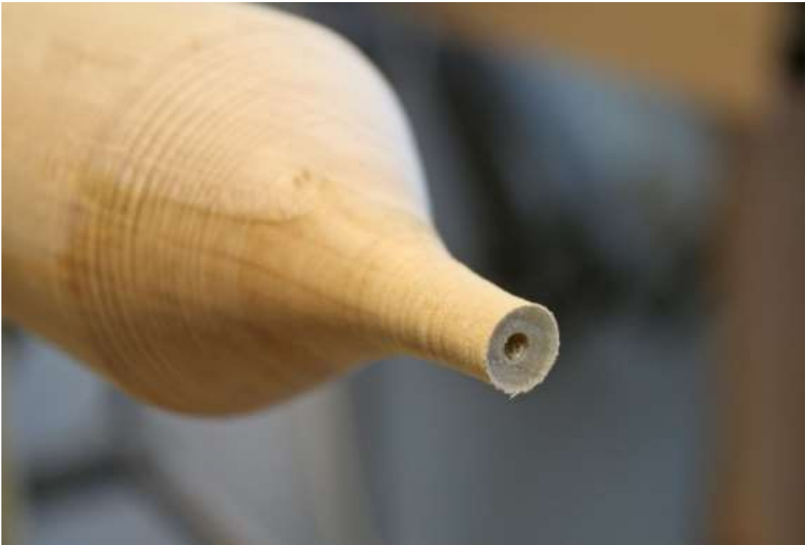
5. end of the cylinder scooped out and hole drilled
