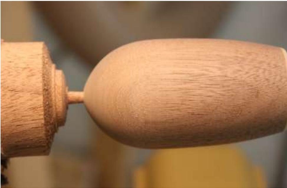
I've rounded the base and sanded it. Note that I've left a large enough gap so I can sand without getting my fingers caught. Also note I've left a small, 1/8" diameter tenon on the goblet. This fits into the 1/8" hole a drilled in the stem to glue the 2 parts together. The tenon is slightly undersized so it'll fit in the hole easily.
