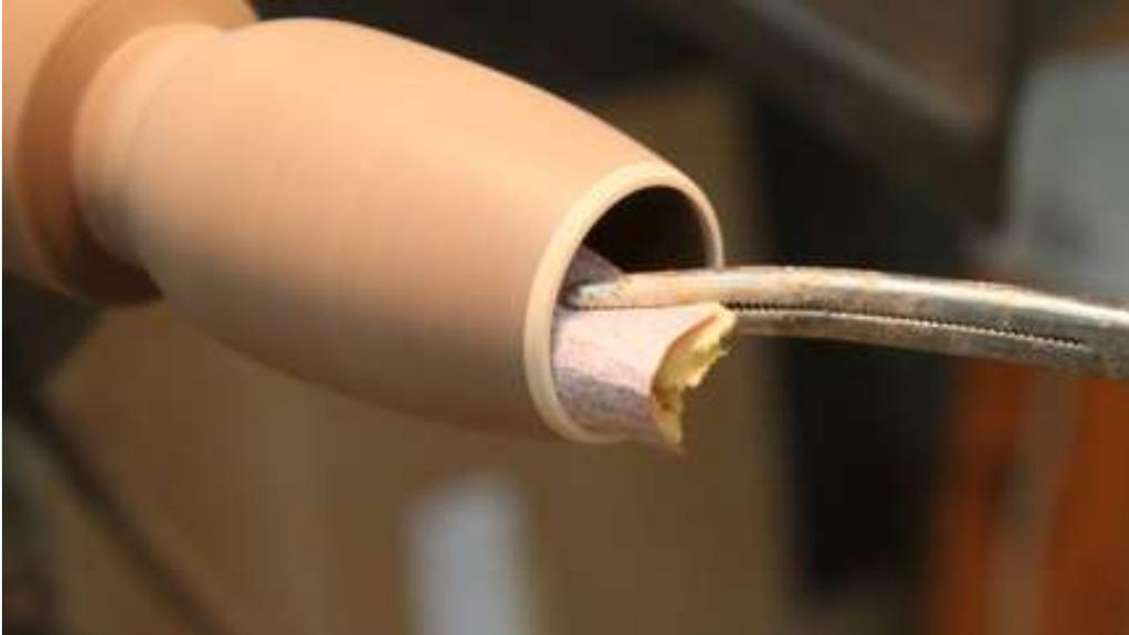
I'm sanding the inside of the goblet using sandpaper on a foam cushion, held in a clamping scissors, like a hemostat.
