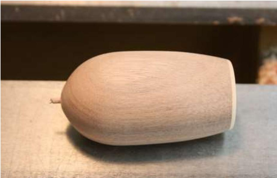
Here the goblet has been parted off and is ready for finish coats to be applied.
