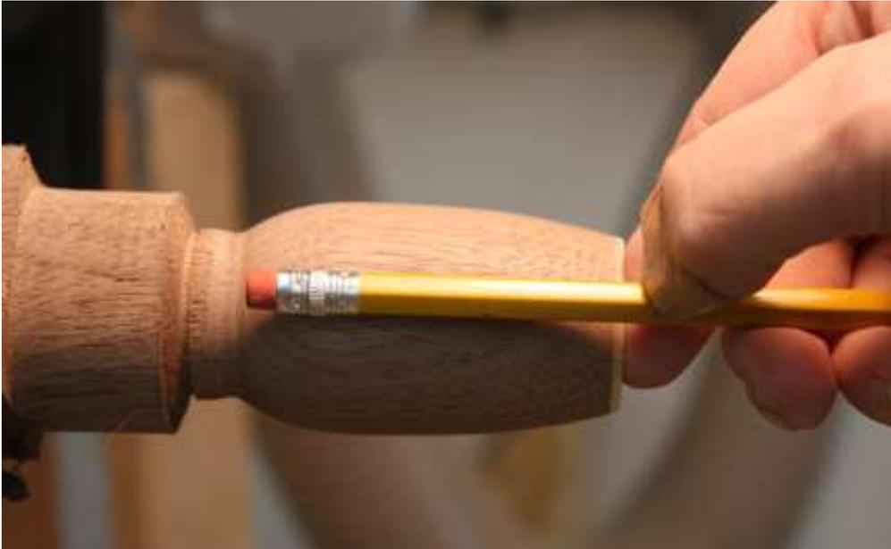
I use a pencil to determine how deep the hole is. I want a little mass left in the bottom so I have enough wood available to round over the outside without cutting through. Like that ever happens!
