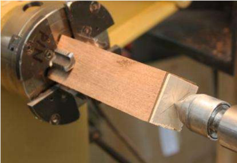
To begin with, I mount a blank in a 4 jaw chuck. The blank has been cut a couple of inches longer than the finished goblet to allow room to work on the base. I've also glued a thin square of maple to the end to make a contrasting rim. Note that I've marked the center of the blank so that the rim will be of a consistent thickness as it's turned.
