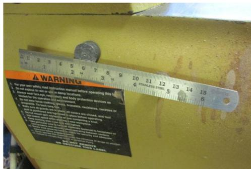
A 1/2 inch magnet will also keep the chuck key handy. Use epoxy or CA glue to secure the magnet to the lathe.
