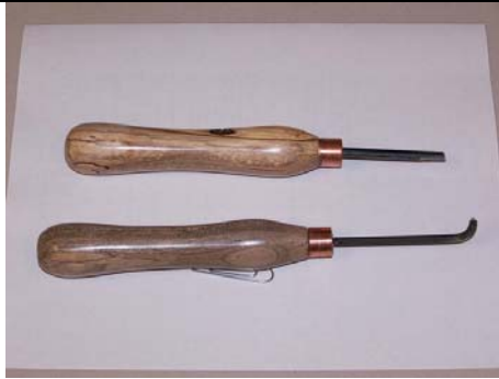
Jim's hollowing tools made from allen wrenches
