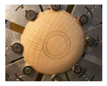
I've added a set of grooves and lines. The grooves are an incised detail and the lines mark the area that'll be textured. I use a parting tool ground down on the sides to make it very thin, around 1/32", where it enters the wood. You can use a skew instead, but there's less chance of the tool catching and skating along the surface with the thin parting tool. The parting tool makes a straight-walled channel instead of a v-shaped one, so if I do any sanding, the grooves will stay the same width.
