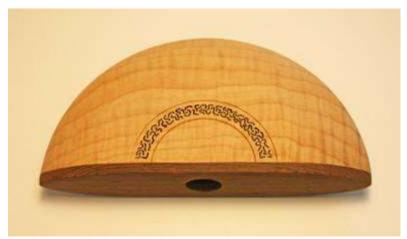
The top has been glued to the vessel and the edges sanded smooth. It's important to not sand too aggressively and sand away any details. The base is held to the vessel with a 1/8" brass pin epoxied in holes drilled in both the base and the center of the vessel. To find the center, I wrap a cloth tape measure around the outside curve of the vessel and divide the measurement by 2.
