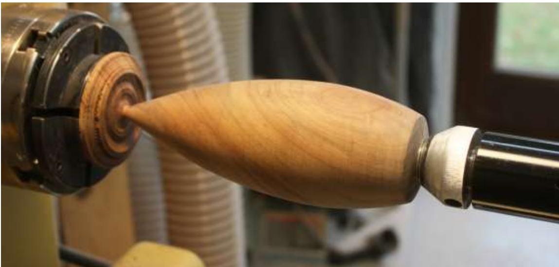
Vessel mostly turned and hollowed, ready to have holes drilled
