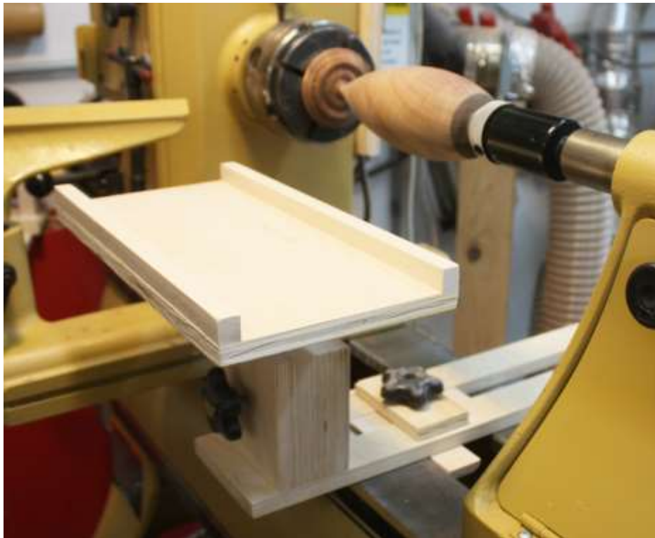
Platform mounted on lathe. Note that it can slide in and out depending on the diameter of the turning.
