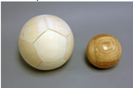
Segmented Balls with no endgrain showing
