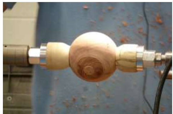
Mounted between jam chucks allows rotating the sphere for final shaping and sanding.
