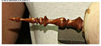
He spent some time showing us how to use our tools to get getter cuts. He uses a parabolic curve on the bevel of his spindle gouge and got a really smooth surface.
